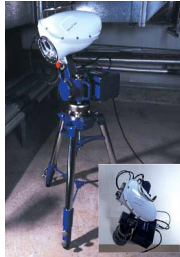
Figure 10. RadScan imaging device (Pajarito Scientific Corporation) [7].
