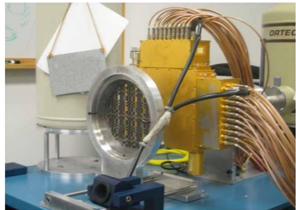
Figure 7. Coded aperture imager. Both the planar and coax detectors are cooled by liquid nitrogen. The coax detector was not used for image acquisition.
