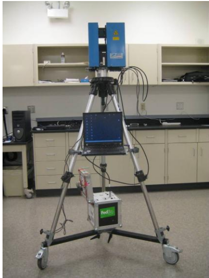
Figure 1. Portable 3D laser scanning system. Unit used in 2006 and 2008 to conduct preliminary tests in laboratory.
