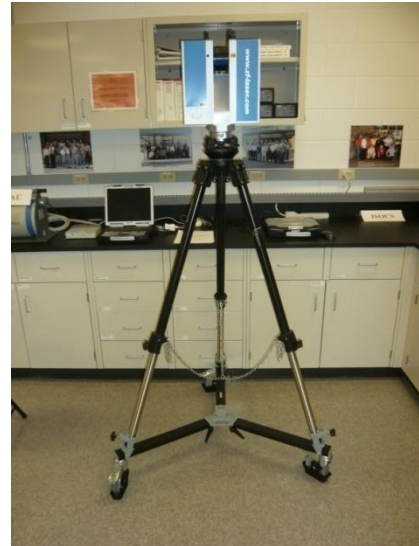
Figure 2. New model of 3D laser that will be used to complete the project. Battery is now part of the single unit, which also stores the image.
