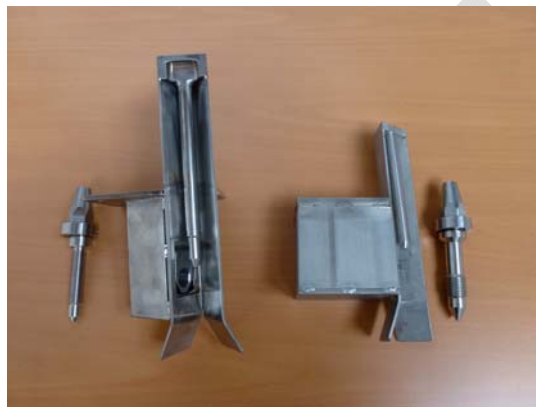
Figure 8 – Locking mechanism (new on the left and first model tested in CNA1 on the right)
