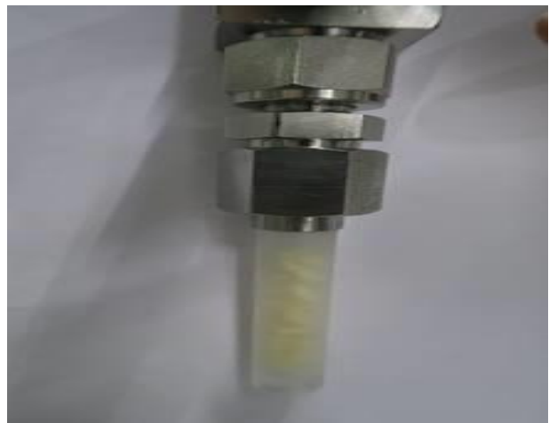
Figure 2 – P10 tube with Al_2O_3 pellets after the reaction with UF_6
