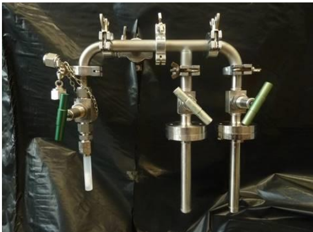
Figure 1- UF_6 sampling rig
