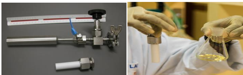
Figure 1: Sample vessels and alumina pellets
