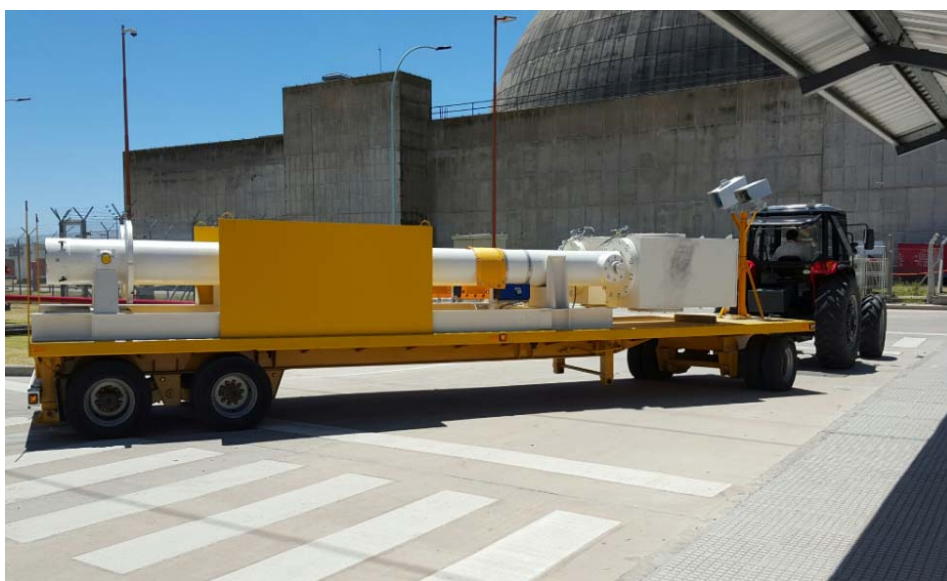
Figure 4: The trailer for flask transfer with surveillance and MUND detector
