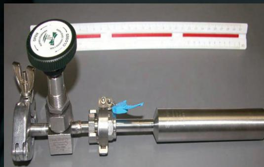
Left: the ampoule currently used for the collection of UF<sub>6</sub>. Right: the material used for collection and transportation by the "ABACC-Cristallini" method.
