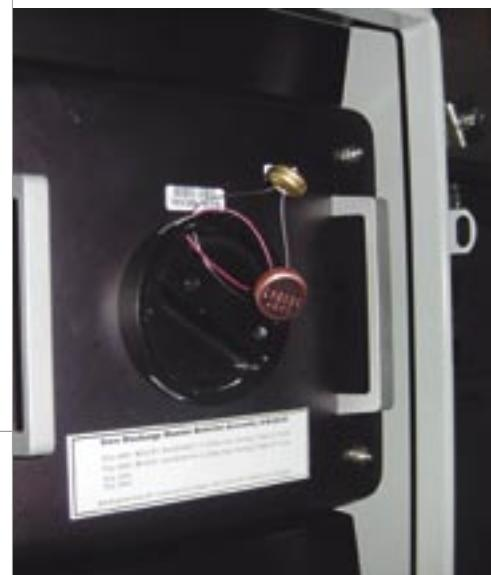
Detector Core Discharge Monitor
