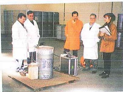
ABACC Inspectors measuring UO<sub>2</sub> drums with NaI detector.
