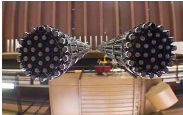
Fig. 1. Atucha-I fuel assemblies.
