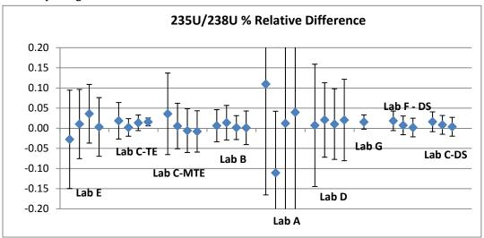
Figure 1: Relative Differences n(U235)/n(U238) ABACC-Cristallini and Hydrolysis methods for each UF<sub>6</sub> CRM
